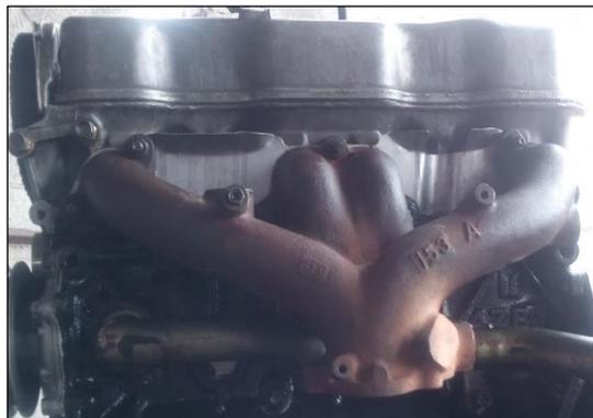
**Figura 3-3:** Colector de Escape
