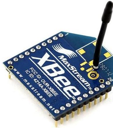
**Figura 18-2:** Xbee S2
