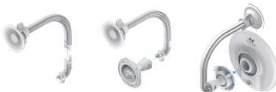
Installation Using the NanoBeam Window Mount
