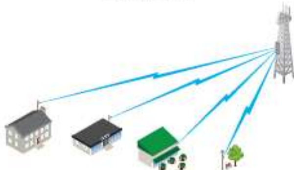
The NanoBeam used as a CPE device for each client in an airMAX PIMP network.
