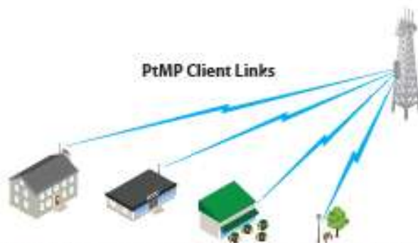
NanoStationM used as powerful clients in an airMAX PtMP (Point-to-Multi-Point) network setup.
