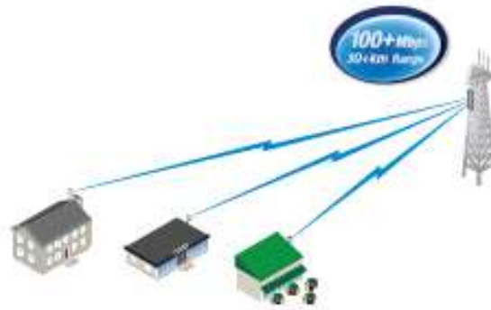
airGrid M as a cost-effective CPE in an airMAX Point-to-Multi-Point network.
