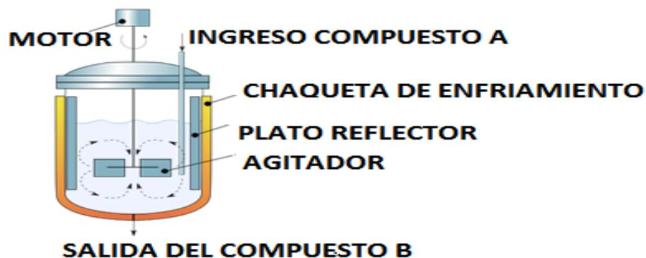
**Figura 1-2.** Reactor CSTR experimental.
