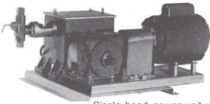
Single head power unit with 10:1 gear reducer for volumes down to 1/4 pint per day. Weight 90 pounds.
