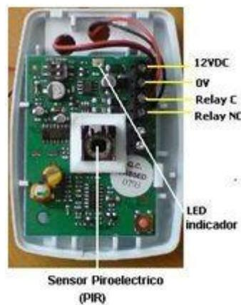
**Figura 10-1:** Tarjeta de control sensor PIR
