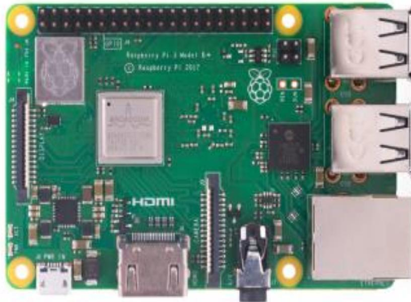
The Raspberry Pi 3 Model B+ is the latest product in the Raspberry Pi 3 range, boasting a 64-bit quad core processor running at 1.4GHz, dual-band 2.4GHz and 5GHz wireless LAN, Bluetooth 4.2/BLE, faster Ethernet, and PoE capability via a separate PoE HAT
