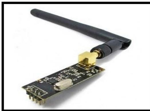
**Figura 4-2:** Módulo NRF24L01
