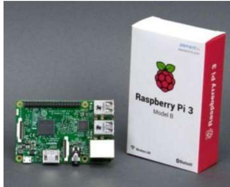
**Figura 6-2:** Raspberry Pi 3, modelo B.
