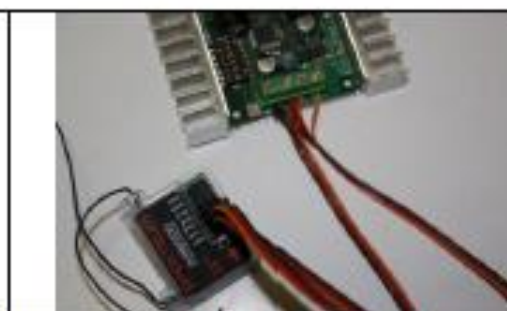
Figure 2.2: R/C input using a receiver powered from terminal 5V
