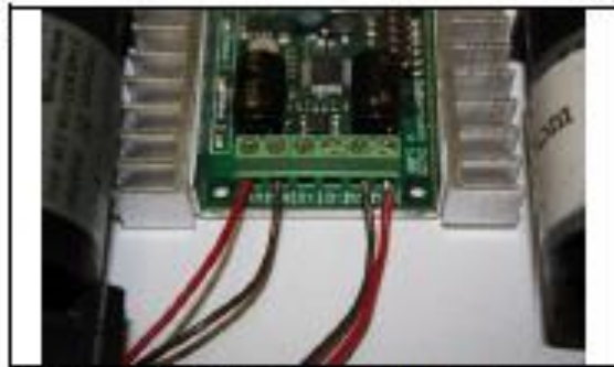
The motors connect to terminals M1A/B and M2A/B
