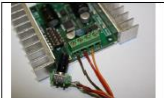
The input signals connect to terminal S1 and/or S2
