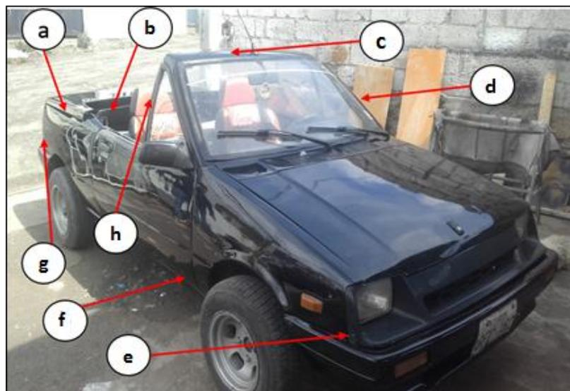
**Figura 7-2:** Paneles exteriores
