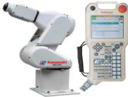
Figura 3. Robot Industrial RS03N y Teach Pendant
