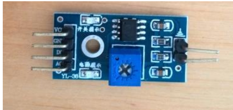
Figura 13-2 Circuito de Control Sensor HL-69
