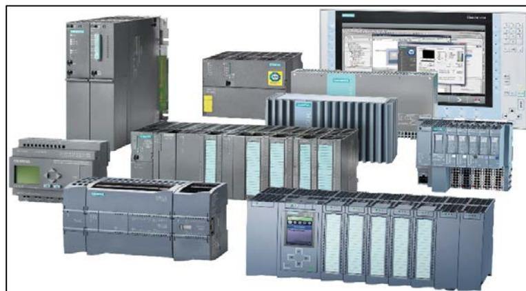
**Figura 5-2:** Modelos PLC (Siemens AG)
