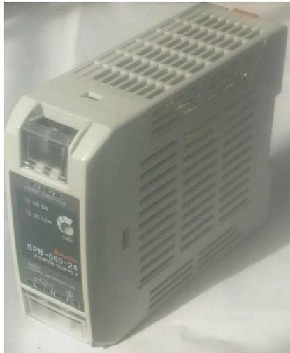
**Figura 10-2** Fuente Autonics 24VDC
