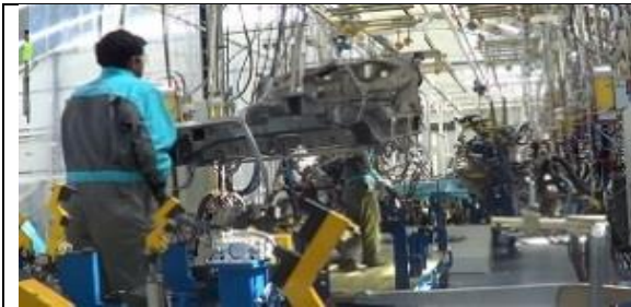
Figura 13-3: Transporte de JIG 1 a JIG 2
