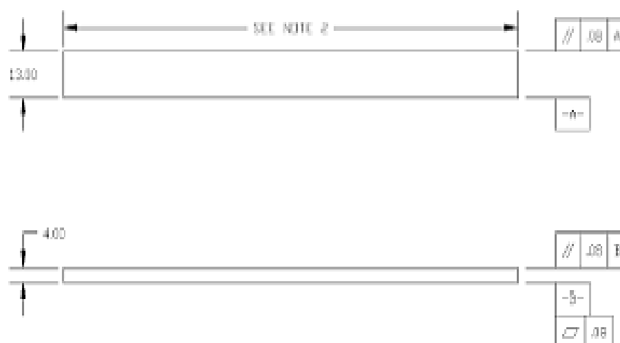
FIG. 4 Standard Flexural Test Specimen Drawing (SI)
