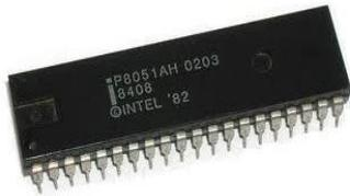
A black integrated circuit (IC) with 40 pins, labeled 80C51AH 0203.   |
