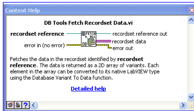
Figura III.91. Icono DB Tools Fetch Recordset Data. Fuente: Manual Labview Database Connectivity Toolkit.
