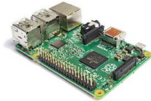
Figura 13-2: Modulo Raspberry Pi
