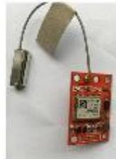
GY-NEO6M-V2 board features the u-blox NEO-6M GPS module with an external antenna and built-in EEPROM. This is compatible with various flight controller boards designed to work with a GPS module.
