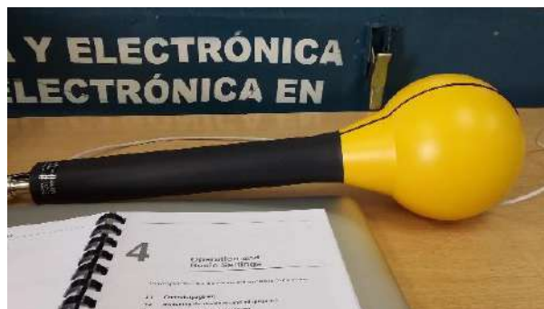
Figura 2-2: Antena de campo E (27 MHz a 3GHz)
