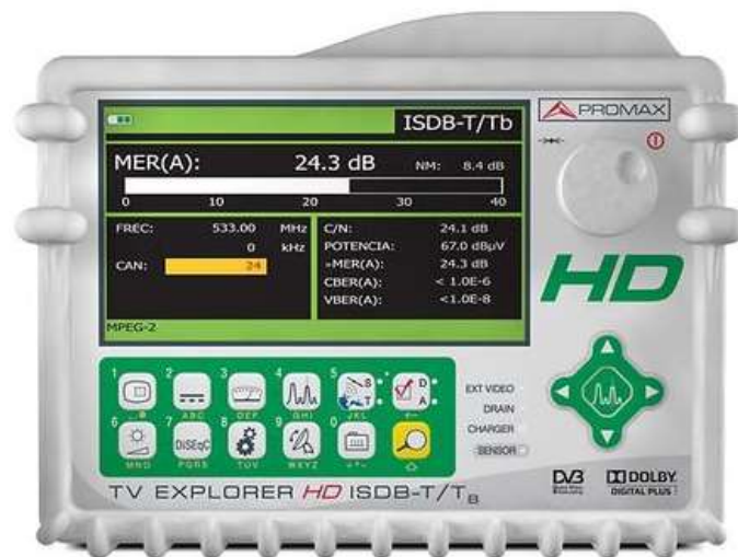
Figura 21-4. Receptor TV Explorer HD ISDB-T/Tb.
