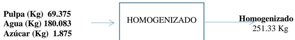
$$\text{Homogenizado(Kg)} = \text{Pulpa (Kg)} + \text{Agua (Kg)} + \text{Azúcar (Kg)}$$
