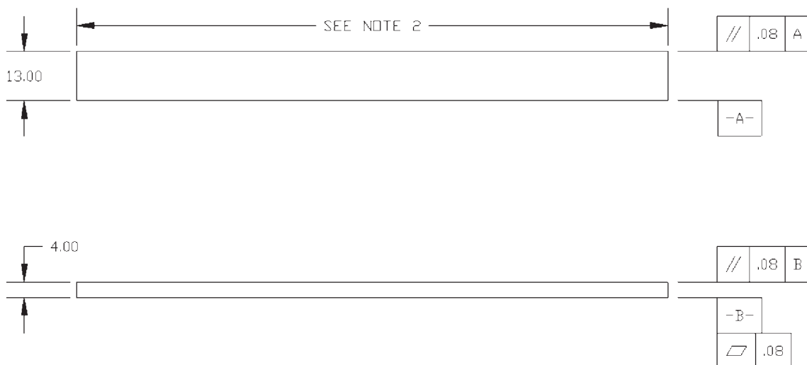
FIG. 4 Standard Flexural Test Specimen Drawing (SI)
