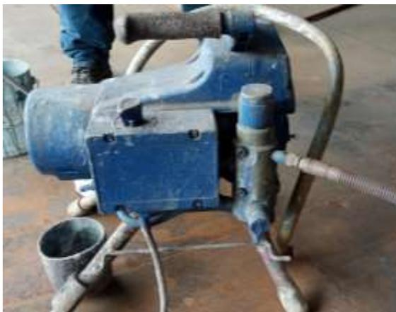
**Figura 13-2:** Bomba Airless Graco ST MAX II 495 PC Pro-17E871
