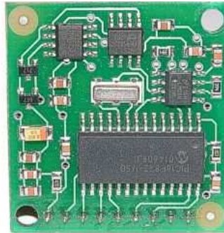
Figura III.18: Brújula digital CMPS03, SUPER ROBOTICA (29).
