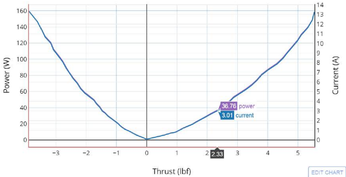
T100 Thruster: Power and Current vs. Thrust
