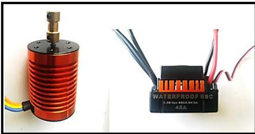
**Figura 9-2: Motor brushless y ESC de 45A.**
