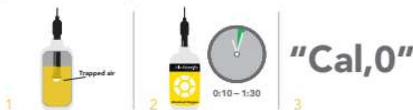
1. Stir probe in Zero D.O. calibration solution to remove trapped air, *(which could cause readings to go high)*.
