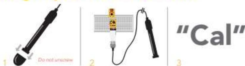
1. Pull off and discard cap from the Dissolved Oxygen probe. *(only used to protect probe during shipping)*
