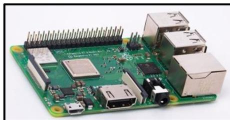
**Figura 11-1:** Raspberry Pi 3 Model B+
