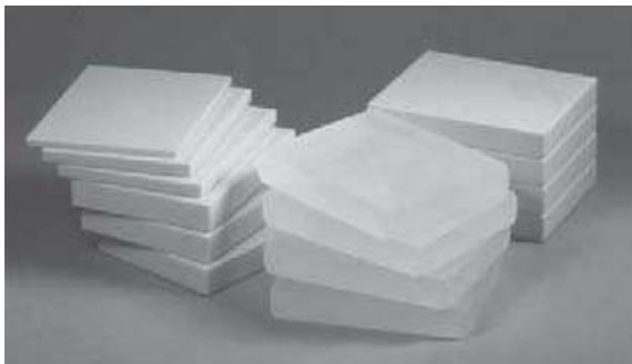
**Modelo:** 18-203 (Mammography Phototimer Consistency Test Tool, set of four acrylic slabs (10 x 12.5 x 2 cm thick). Weight: 3 lb (1.34 kg)).
