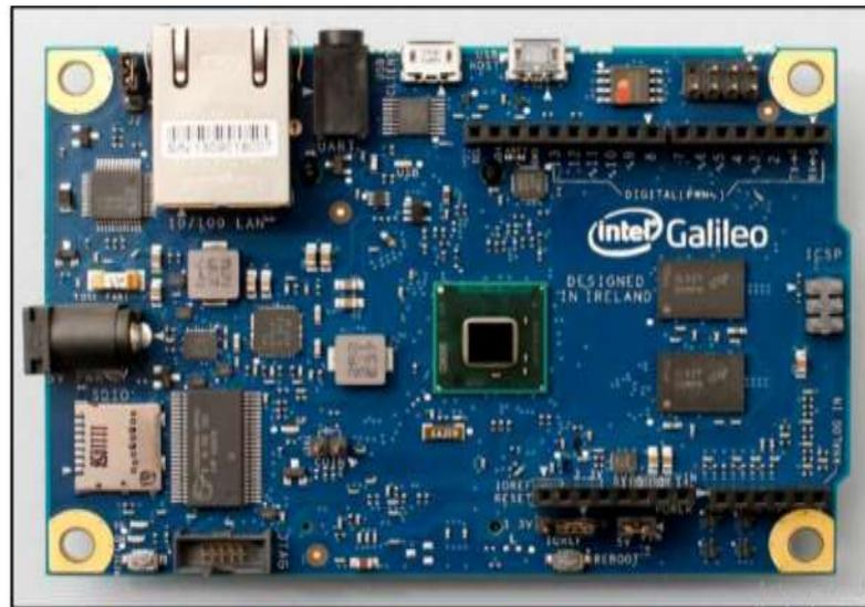
Figura 4-1 Tarjeta Intel Galileo
