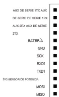
**Figura 17-2:** Pines de conector SPI-UART
